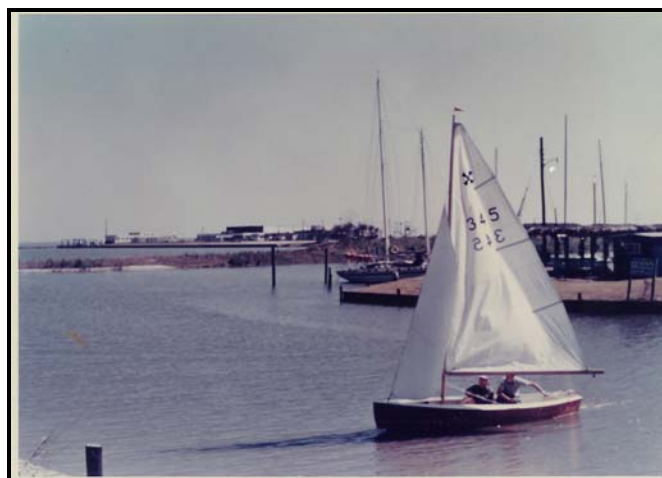
Dr. Sam Showalter built a Windmill while in high school with a varnished mahogany hull, slotted spruce mast, and homemade stainless hardware. This photo was taken in about 1962. Note the PAYC Aloha Hut on the right and the Pleasure Pier swimming pool and ballroom in the background on the left.
